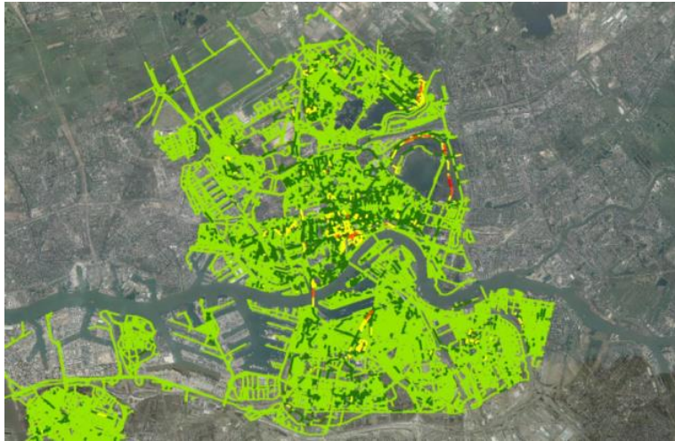
Figure 1. Green shows high positional accuracy, red is poor positional accuracy due to minimal GPS/IMU signal under urban canyons and dense vegetation.
